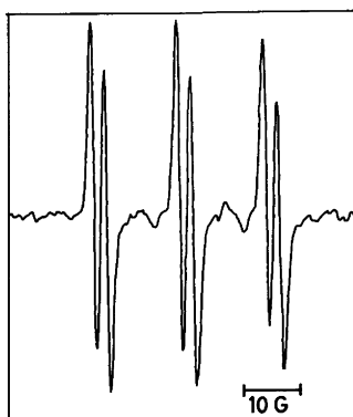
Fig. 1. ESR spectrum obtained in the reduction of \text{CCl}_4 with \text{CoW}^{7-} in the presence of PBN.
