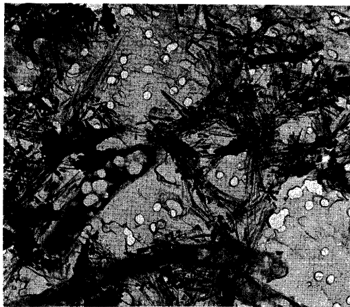
Fig. 10. NaAlF 4 fibers contained in distilled water for 97 h at 20°C. TEM 8400×.
