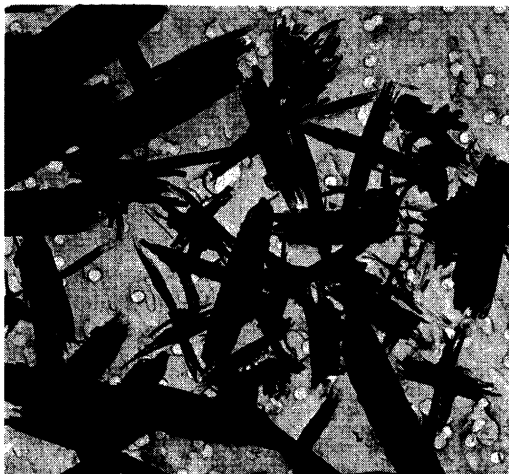
Fig. 9. NaAlF 4 fibers contained in distilled water for 24 h at 20°C. TEM 8400×.
