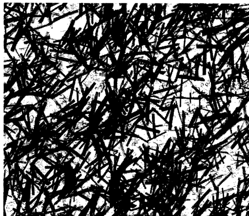
Fig. 3. \text{NaAlF}_4 fibers grown at flow rate 15 \text{ dm}^3/\text{h} ( 810^\circ\text{C} ). TEM 3100\times .
