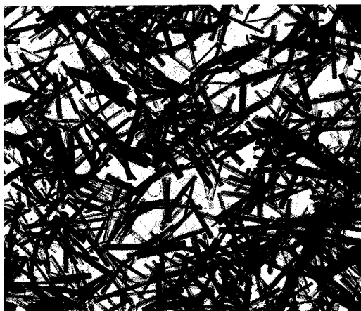
Fig. 2. \text{NaAlF}_4 fibers grown at flow rate 12 \text{ dm}^3/\text{h} ( 810^\circ\text{C} ). TEM 3100\times .
