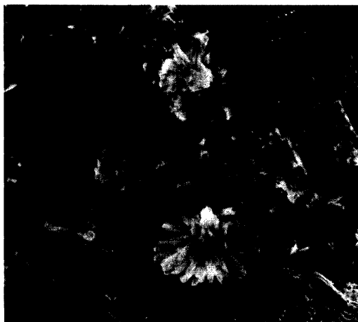
Fig. 5. \text{NaAlF}_4 particles (same sample as in Fig. 4) photographed in SEM 9000 \times .
