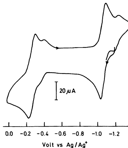
Fig. 3. Cyclic voltammogram for m -chloronitrobenzene following coulometric reduction at -1.12 V. Sweep rate 200 mV/s. C=4.1 mM, t=-40 °C.
