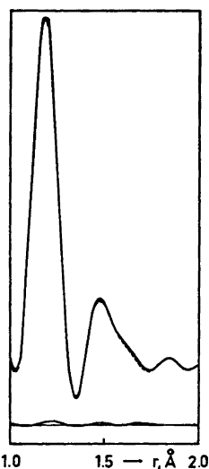
Fig. 5. Fumaraldehyde. Experimental (—) and theoretical (---) autocorrelation power spectra. Antidamping constant \alpha = 0.04 . \tau_{\max} = 30.0 \text{ \AA}^{-1} .
