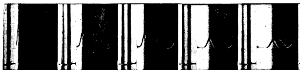
Fig. 5. Schlieren diagram of the ultracentrifugal sedimentation of the purified preparation of cytochrome c peroxidase. The concentration of the enzyme was 3.23 mg/ml in a buffer of pH 7.0, \mu=0.283 , 0.05 M in sodium phosphate and 0.171 M in sodium chloride. The photographs were taken at a phase angle of 45° 8, 24, 32, 56, and 72 min after 59 780 rpm were reached at 20°C. The sedimentation is from left to right.
