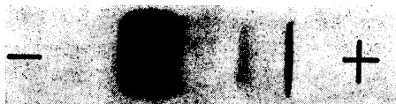
Fig. 2. Urea-starch gel electrophoresis of three times crystallized lactoferrin. The electrophoretic run was performed in 0.035 M sodium formate buffer, pH 2.8, for 7 h at 8 V/cm. 13
