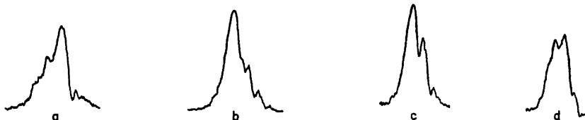
Fig. 3. Results of the selective double irradiation experiments in 2,3-dimethylthiophene; (a, b) and (c, d) show the low field part of the 4-hydrogen band for selective decoupling of J_{(\text{CH}_3)2-4} and J_{(\text{CH}_3)3-4} , respectively. The corresponding positions of the decoupling rf. field are indicated by arrows in Fig. 1a.
