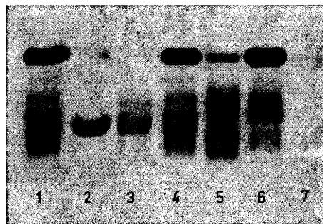
Fig. 1. Electropherogram of plasma and fractions. The electrophoresis was run on cellulose-acetate strips at pH 8.6, 300 V and 4–7 mA for 20 min. The apparatus used was a Beckman model R-101 microzone electrophoresis cell (Beckman instruments, California). A barbital buffer (Beckman B-2), pH 8.6 and ionic strength 0.075 was used. Fractions A I–A III and fraction A V were dissolved in a volume of one fourth and fraction A IV in a volume of one half that of the starting plasma. 1 and 4. Plasma (0.25 \mu l). 2. Fr. A I (0.25 \mu l). 3. Fr. A II (0.25 \mu l). 5. Fr. A III (0.25 \mu l). 6. Fr. A IV (0.5 \mu l). 7. Fr. A V (0.25 \mu l).
