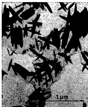
Fig. 1. Electron micrograph of precipitate from slightly hydrolyzed 10 mM Fe(III) in 0.5 M NaCl solution.
