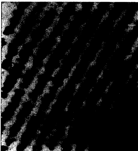
Fig. 2. Section of coating, magnification 40 000, dry state.
