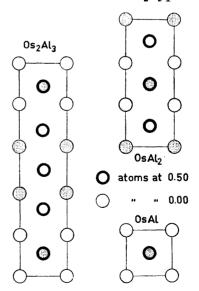
Fig. 1. The unit-cells of OsAl, Os<sub>2</sub>Al<sub>3</sub>, and OsAl<sub>2</sub>. The osmium atoms are dotted.
