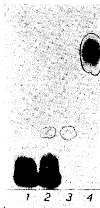
Fig. 2. Paper chromatogram of hay extracts and ascorbigen preparation 5 in Fig. 1. Solvent and spraying solution as in Fig. 1. 1. Extract prepared from 200 mg of the hay used in the experiments with guinea-pigs. 2. Hay extract + 2 \mu g of ascorbic acid, 3. 2 \mu g of ascorbic acid, 4. 1 mg of ascorbigen prepared from 3-hydroxymethylindole and ascorbic acid.
