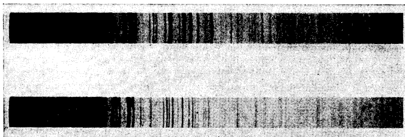
Fig. 5. X-Ray powder diagram of HserP from L. casei (upper) and synthetic HserP (below). Guinier camera. Nickel-filtered copper K -radiation.
