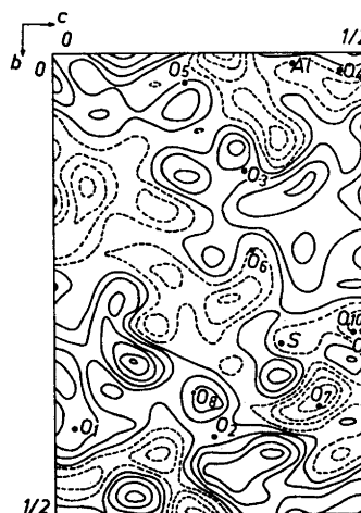
Fig. 3b. F_0 - F_c synthesis along [100] . Contours are drawn at intervals of 0.3 e \cdot \text{\AA}^{-2} . Dashed lines indicate negative regions.
