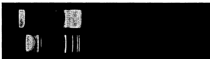
Fig. 3. X-Ray powder diagram of the dephosphorylated compound (below) is identical with that of muramic acid (above). (Some impurity in muramic acid has given a few additional weak bands.)
