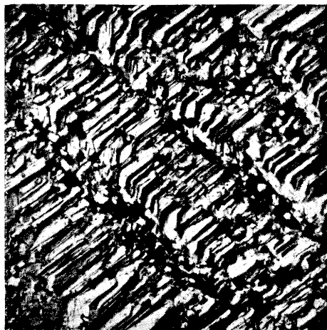
Fig. 12. Oxide surface of Kroll titanium oxidized for 10 min at 890°C and p_{O_2} = 1 atm. 3 500 \times .
