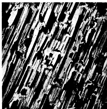
Fig. 13. Oxide surface of Kroll titanium oxidized for 60 min at 890°C and p_{O_2} = 1 atm. 8 200 \times .
