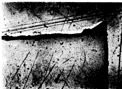
Fig. 19. Van Arkel titanium oxidized for 5 h at 700°C. 375 ×.
