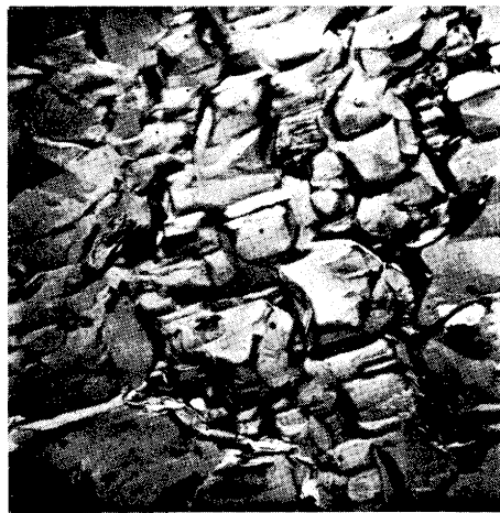
Fig. 15. Oxide surface of Kroll titanium oxidized for 10 min at 1 000°C and p_{O_2} = 1 atm. 3 500 \times .
