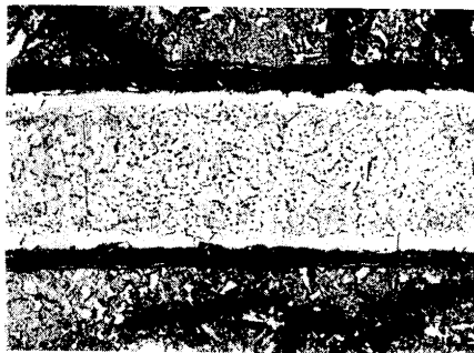
Fig. 21. RC-55 titanium oxidized for 5 h at 825°C. 75 \times .
