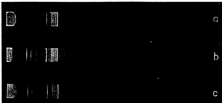
Fig. 1. X-Ray diffraction patterns of sialic acids isolated from (a) human, (b) hog and (c) horse kidneys.
