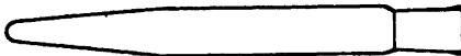
Fig. 1. The vessel in which all operations take place. It is furnished with a standard taper female joint 10/15. Total length: 116 mm, max. diameter: 12 mm, volume up to the joint: about 7 ml.
