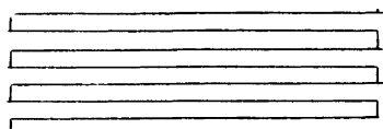
Fig. 8. Recording of step-wise resistance changes of 100 ohms at a recorder range of 200 ohms. Paper speed 5.9 mm per minute.
