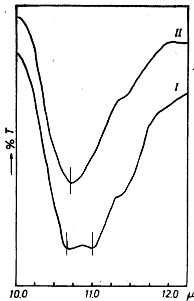
Fig. 1. I: Racemic \alpha,\alpha' -dimethylglutaric acid in chloroform solution. II: (+)- \alpha,\alpha' -dimethylglutaric acid in chloroform solution.
