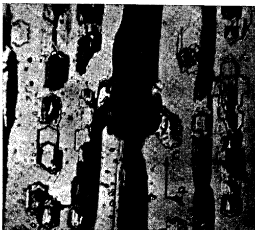
Fig. 5. Different types of etch-pits. 3 C H 2 SO 4 , 8 min at 100° C. Refl. light, one Nicol, magn. 230 x. (Phot. Brotzen.)
