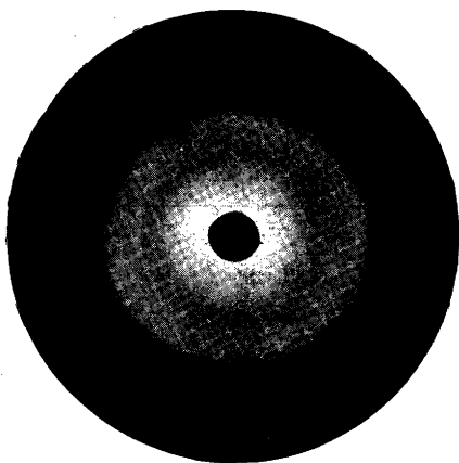
Fig. 6. X-ray diffraction diagram of charcoal-sulphur compound (approx. 13 % S). The preparation has been heated and then extracted with hot aniline.
